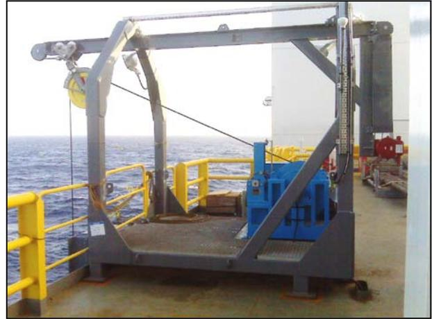
Velocity measurements are made by a Teledyne RD Instruments (TRDI) Long Ranger, a 75 KHz Acoustic Doppler Current Profiler (LR75 ADCP). The LR75 is mounted on a steel sled, which rides between the deck and the operational position at the turn of the bilge keel along steel rails mounted to the hull.
